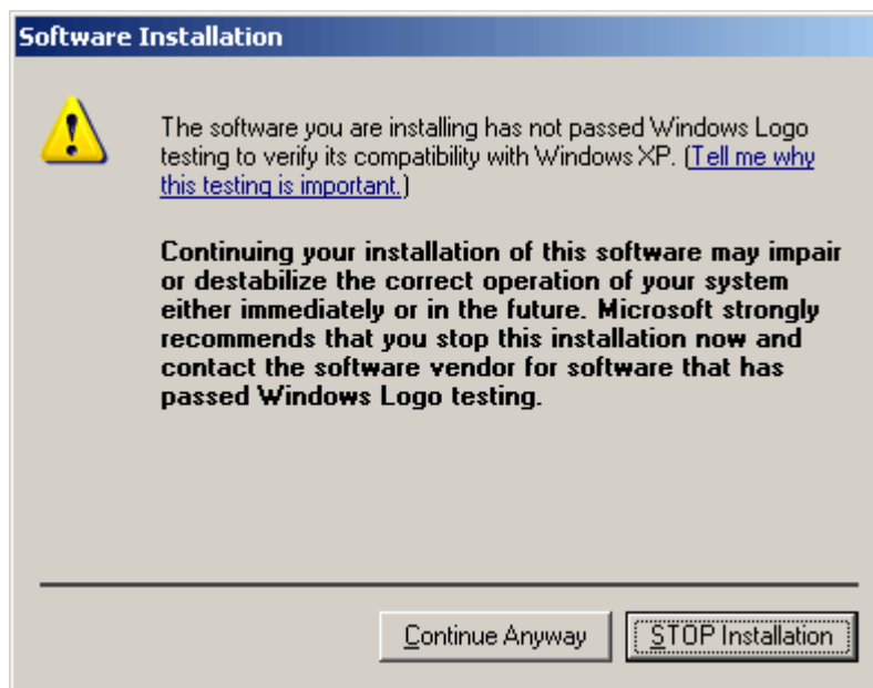
Figure 15 - Windows Logo Testing dialog box. Click 'Continue Anyway' if this is shown.
